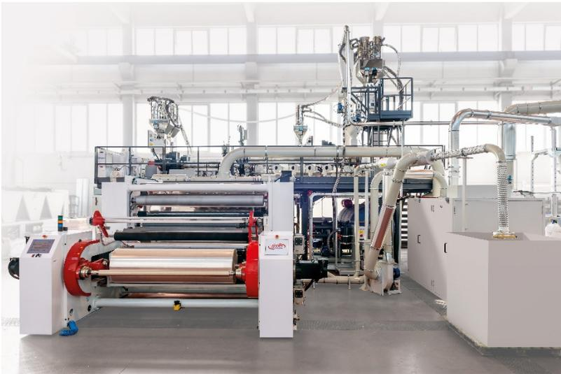
This line is considered a flagship project in this field also for having a 4-layer multi manifold die which allows an extremely accurate distribution of the layers by using 4 extruders.
